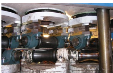
14. Roller straightening force system
